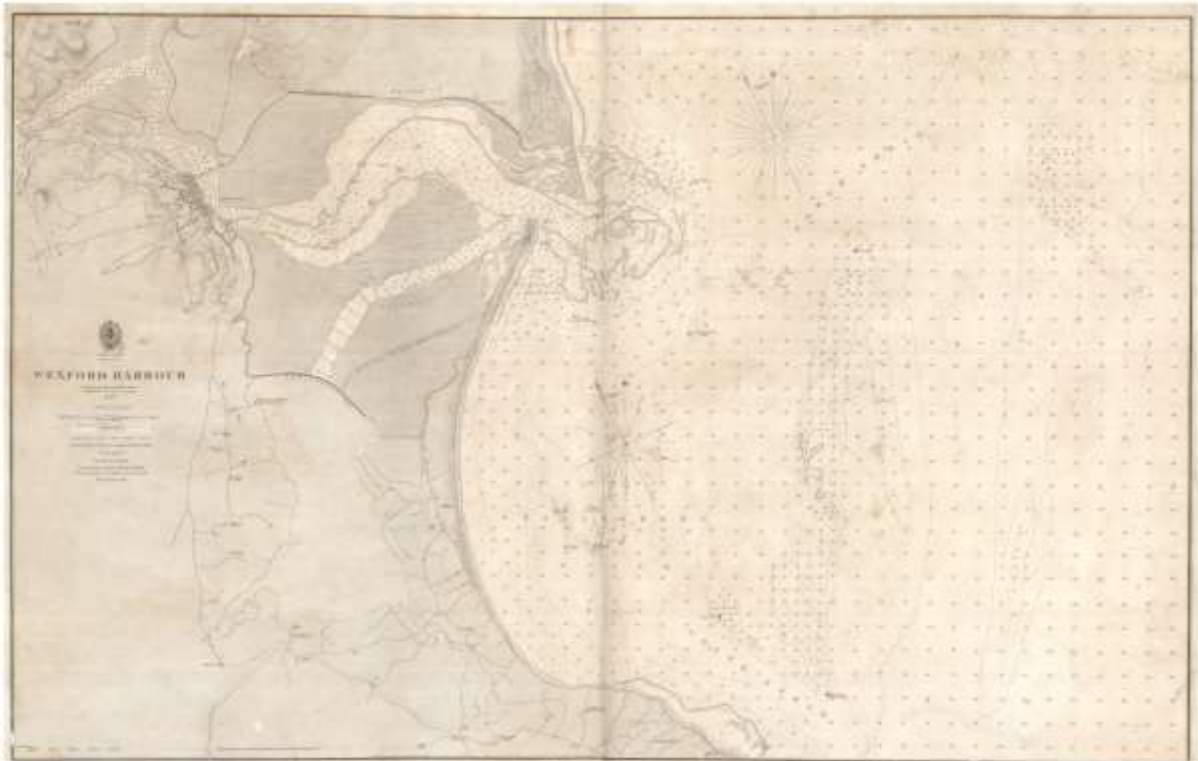
Figure 10: Wexford Harbour Bathymetry by G.A. Frazer of 1845 and corrected by same in 1856 presumably after the embankments for the north and south slobs were built in 1847-1849 and 1853 - 1854 respectively. The Rosslare point ran up much closer to the Raven Point before it was washed away in the early 19 th Century (?)
